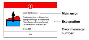
A variety of messages can be displayed. These messages can occur during start up or during counting. The error message screen shows the main error, the explanation and solution and the error message number.
