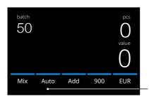
With setting 'Auto'is activated the machine will automatically start count when banknotes are placed on the hopper. With Auto deactivated, the **[START/OK]** button must be pressed to start counting.
