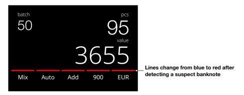
After finishing the count (when the hopper is empty), the device will repeatedly make 3 beep tones and the lines remain red. After removing all the banknotes from the reject pocket, the red line will return to the colour blue.
