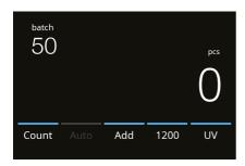
**3.** Place a stack of banknotes on the hopper. The device will now stop counting when the batch number has been reached.
