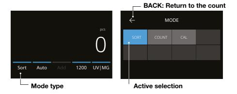
2. The mode menu contains multiple selection tiles. The active mode type has a blue coloured tile. The available mode types are determind by the active detection type. Simply press a mode type you require for your count.
