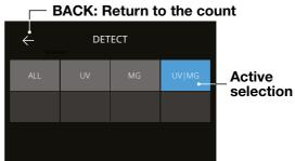
2. The detect menu contains multiple selection tiles. The active detection type has a blue coloured tile. Use [LEFT] & [RIGHT] buttons to toggle between the detect menu pages. Simply press the tile corresponding to the currency or a detection manner you require on the screen for your count.
