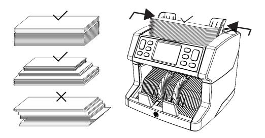
**3.** When the banknotes are placed on the hopper the machine will automatically start counting. Press **[AUTO]** on the screen to switch Off this function.
