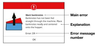
A variety of messages can be displayed. These messages can occur during start up or during counting. The error message screen shows the main error, the explanation and solution and the error message number.
