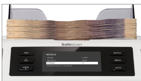
Sheet counting option (free count) without counterfeit detection
