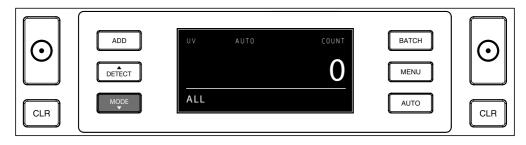
2. AUTO START / MANUAL START. By pressing the AUTO button, you can select whether you want the banknote counter to start counting automatically or manually. When the screen shows 'AUTO', the machine will start counting once banknotes have been placed in the hopper. Default setting = AUTO.
