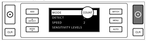
7. After settings have been done, exit the menu by pressing the MENU or the CLR button. The banknote counter will return to the main screen.
