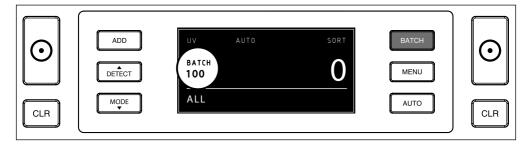
2.2 While the amount is blinking, you can navigate through the preset batch numbers by pressing the **BATCH** button again. The sequence is 100 > 50 > 20 > 10 > 5 > Batch off.
