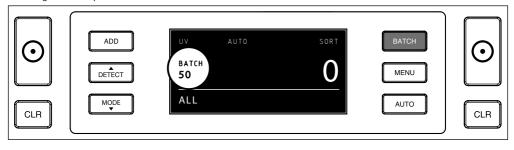
2.3 Use the arrow keys to increase or decrease the batch number 1 piece, starting from the number that is blinking.
