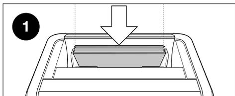
First, place the stack of banknotes facing forward on the hopper (1).
