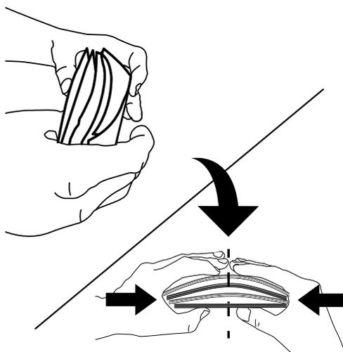
3. Place the stack on the hopper, with the largest banknotes facing up. Then gently push the banknotes back vertically to start counting.
