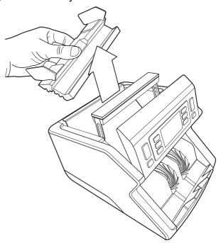
**4.** Clean the sensors and the rotation wheels carefully with a dry brush or air duster
