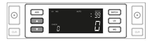
**2.4.** Confirm the batch number by pressing the **START** key. After this, the set batch number will remain visible in the screen.
