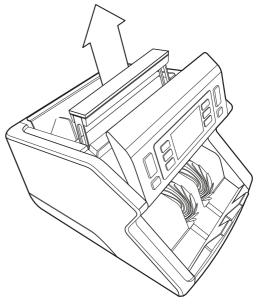
3. Remove the hopper guide assembly
