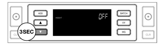
Please note that in this setting the device will not be able to detect banknotes of a different height and/or width when these are included in the counted stack.
