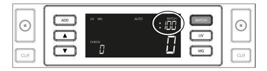
**2.2.** Navigate through the pre-set batch numbers by pressing the **BATCH** button again. The sequence is: 100 > 50 > 20 > 10 > Batch off.
