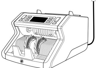
Switch on the banknote counter by pushing the power switch at the back in the "1" position.
