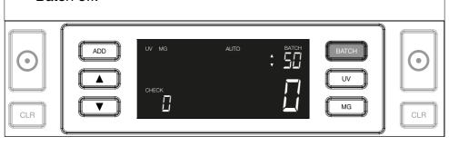
2.3. Use the arrow keys to increase or decrease the batch number by 1 piece, starting from the number that is shown. When the display shows '100', you can go to 101, 102 etc. by pressing and to 99, 98 etc. by pressing
