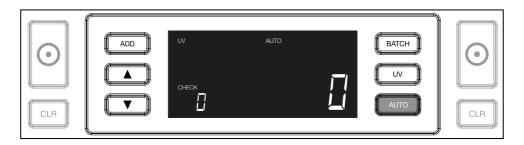
Safescan 2250: press the **START** button for 3 seconds to activate/de-activate the auto start function.
